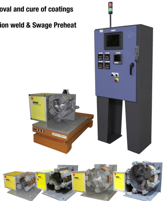
6 Coil diameters cover the complete OCTG pipe range
